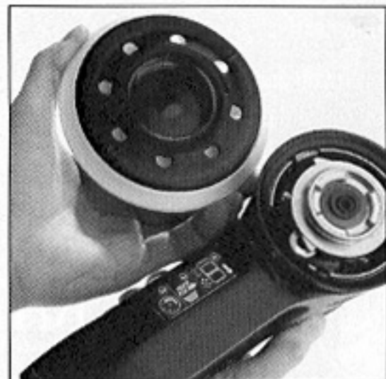
A SPINDLE LOCK allows sanding pads to be changed quickly and easily.
