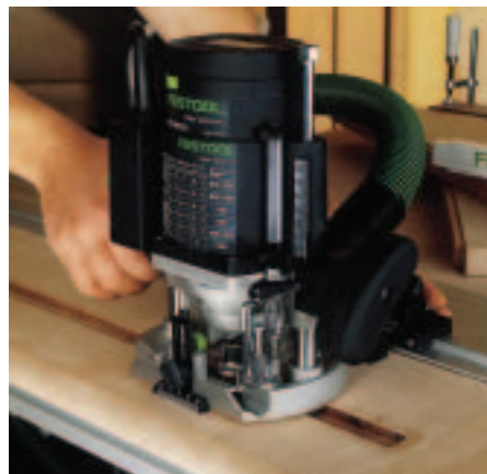
Simple and precise: setting the depth stop.
