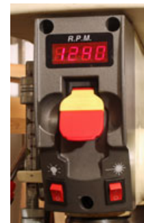
The single speed lever (left) operates the pulleys while the digital display (right) shows the exact spindle speed!
