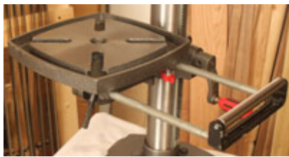
The cast iron table (left) has an extendable roller work support that makes the big jobs easier. The table has a special mount (right) that allows pivoting the table around its center as well as raising and lowering it!
