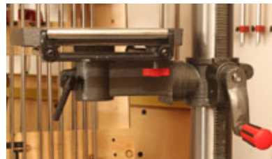
The cast iron table (left) has an extendable roller work support that makes the big jobs easier. The table has a special mount (right) that allows pivoting the table around its center as well as raising and lowering it!
