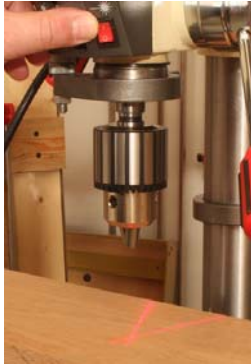
The dual lasers produce a crosshair that makes drilling very precise.
