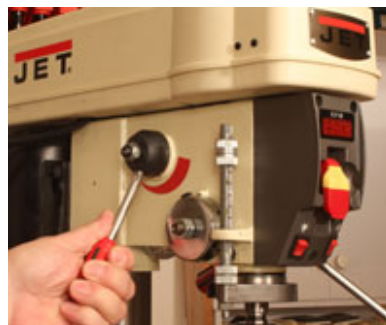
The single speed lever (left) operates the pulleys while the digital display (right) shows the exact spindle speed!
