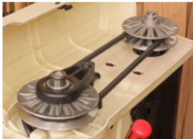
The variable pulley system creates the infinitely adjustable 500 to 3000 RPM spindle speed range.
