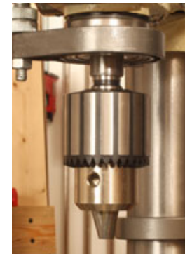
The 5/8"-capacity chuck is mounted to the spindle with a #2 Morse taper.
