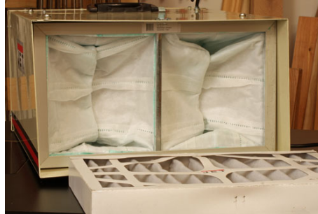
The dual filter elements (left) allow the AFS-400 to capture particles down to 1 micron in size! Both filter elements are easy to remove by simply flipping open the spring-loaded clips (right) and slipping them out of the cavity.
