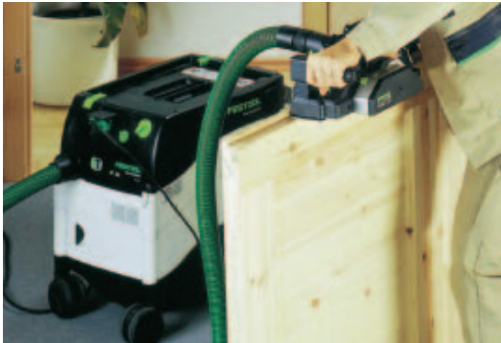
3 15/64" (82 mm) planing width, unlimited rebate depth. Only with the Festool HL 850 E.
